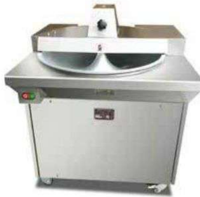
Food Cutter Machine Power: 1500W Bowl Dia: 600mm
